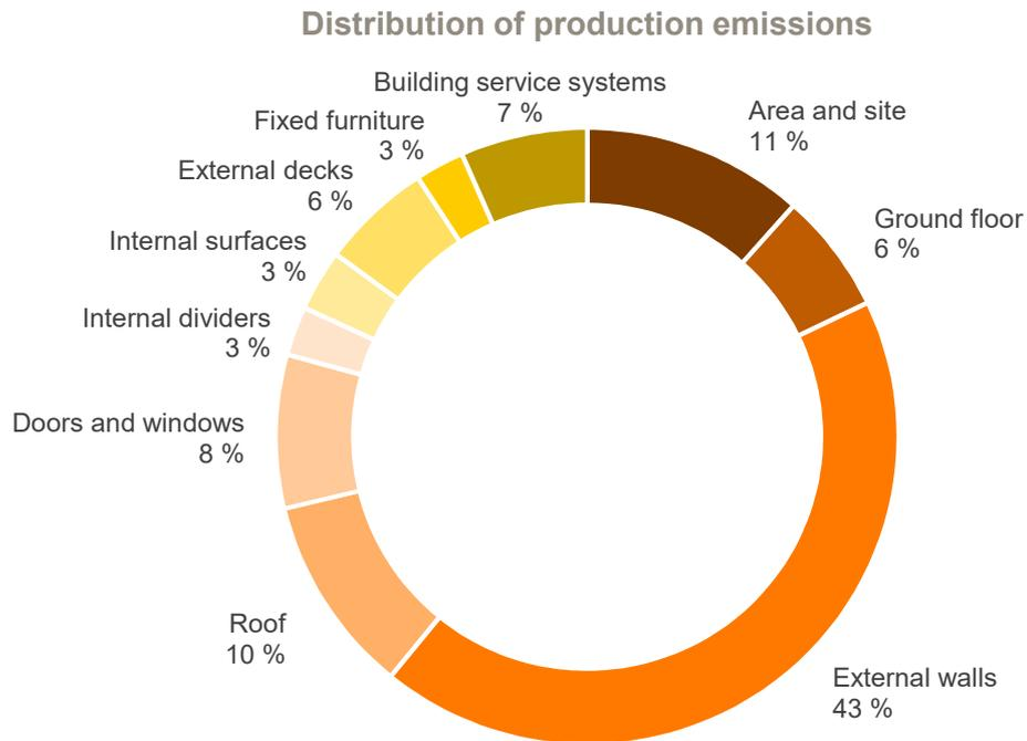
Majority of the emissions are related to the production of the external wall and the loadbearing frame (45%). These building parts include high degree of metals that still have moderate amounts of recycled raw materials. Had they higher recycled scrap content in the future, the emissions from the production of such components would be lower.
