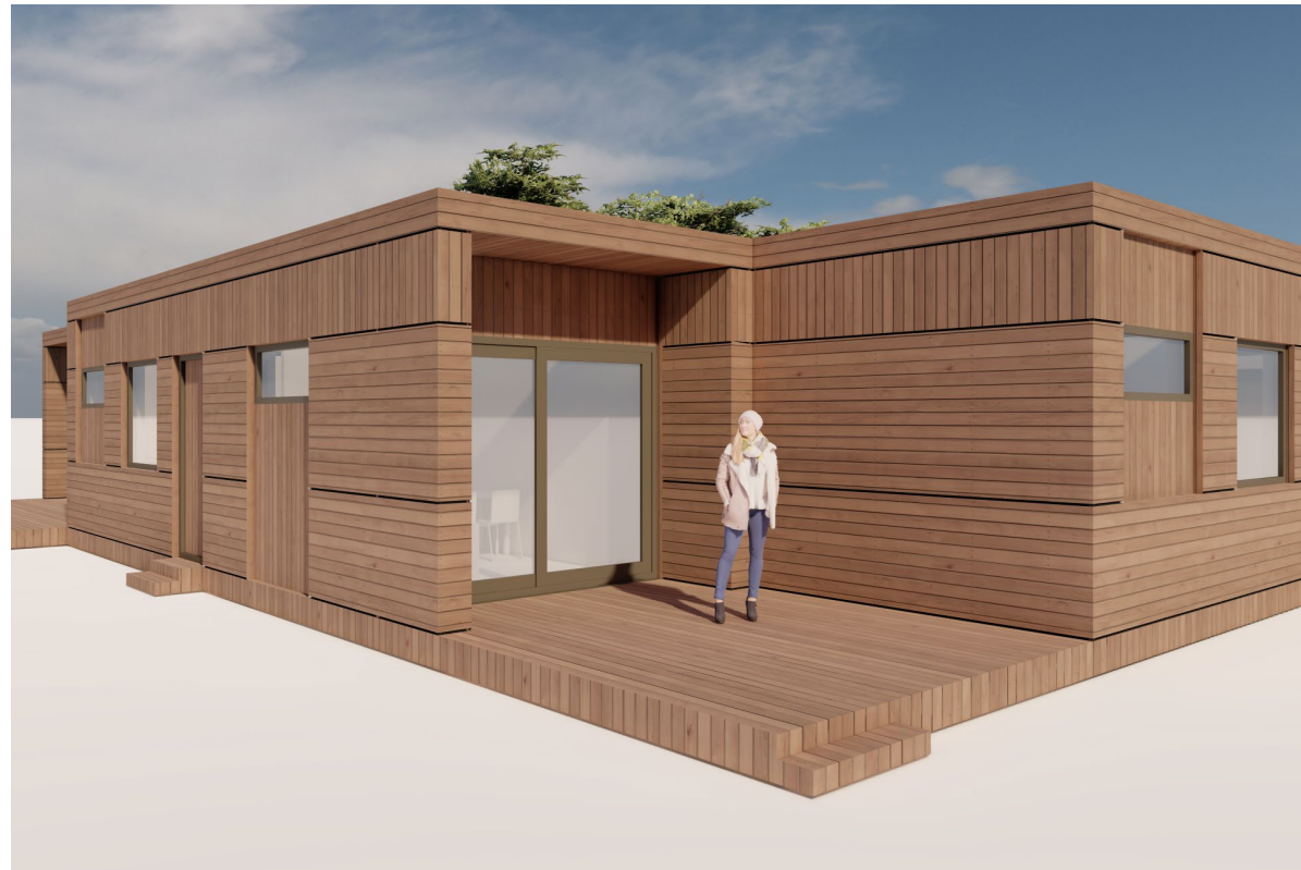
Bamboo Cladding - Comparable to an ordinary wood facade but reducing the carbon footprint Moso Bamboo - Bamboo x-treme cladding
