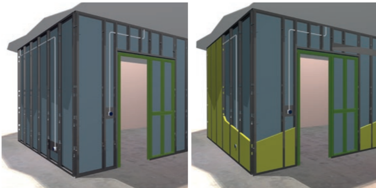
The steel studs are placed in the tracks without separate fastening; they are fixed together during the sheeting process. This facilitates work and also enhances working safety.
